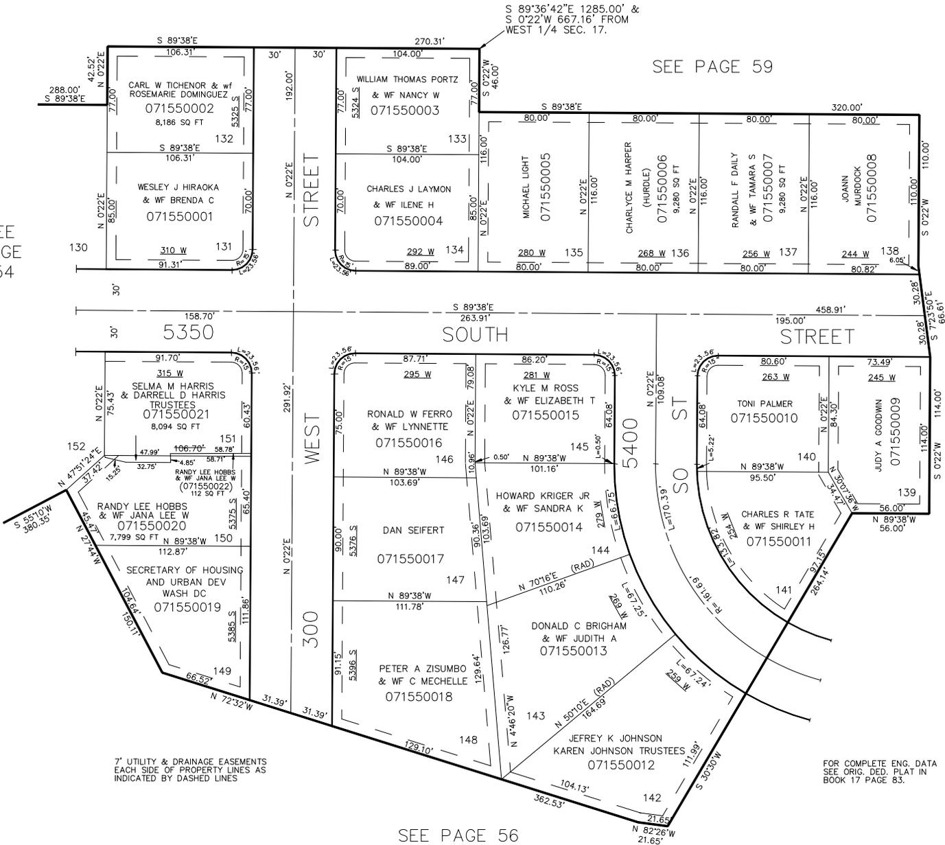
7' UTILITY & DRAINAGE EASEMENTS EACH SIDE OF PROPERTY LINES AS INDICATED BY DASHED LINES
